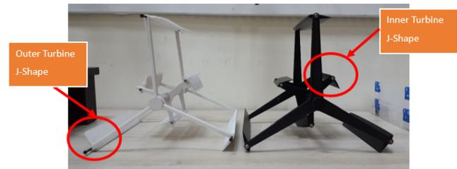
**Figure 13.** C1 and C2 configurations of hybrid VAWT.
